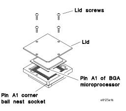
**CAUTION:** Multiple insertions of the BGA microprocessor into the BGA carrier may degrade the ball nest socket connections. Once the BGA microprocessor is inserted in the ball nest socket, tighten the four lid screws forcefully. Only remove the BGA microprocessor from the BGA carrier when necessary for silicon upgrades.
