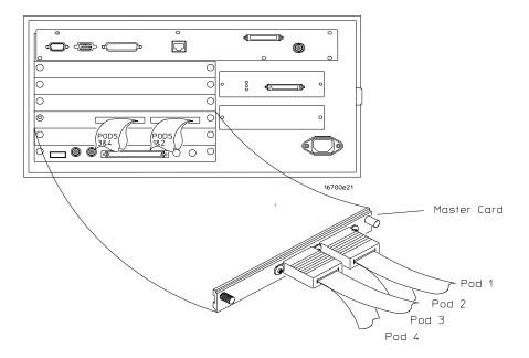
Use this table to connect cables from the logic analyzer to the connectors on the analysis probe or on the target system.
