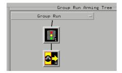
Clicking the **Group Run** button (at the very top of the Intermodule window or a logic analyzer window) will start the analyzer running. The analyzer will then wait for an arm signal. Now, when the emulation module transitions into "Monitor" from "Running" (or from "Reset"), it will send the arm signal to the analyzer. If the emulation module is "In Monitor" when you click **Group Run**, you will then have to go to the emulation module or your debugger interface and manually start it running.
