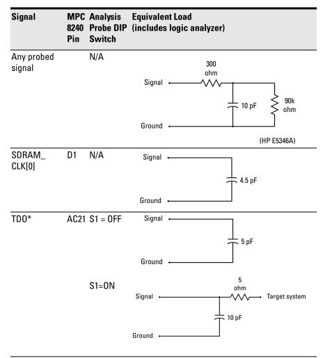
\*Signal is on the JTAG port. The equivalent load does not include the emulation module /probe.
