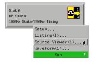
The source correlation tool set correlates the logic analyzer's address label with a line of high-level source code whose address, symbol name, file name, and line numbers are described in a symbol file downloaded to the logic analyzer (see "To load object file symbols" on page 128).
