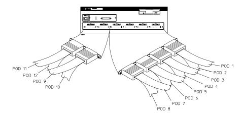
Use this table to connect cables from the HP 16600A logic analyzer to the connectors on the analysis probe or on the target system.
